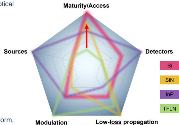
Fig. 1. Properties of various PIC platforms.
