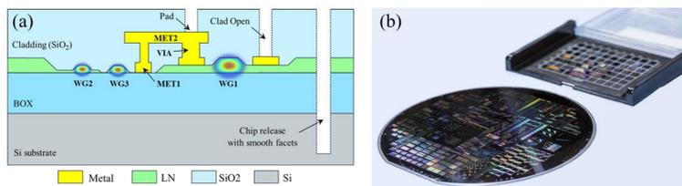
Fig. 3. (a) Schematic of the TFLN PIC platform's technology cross section, (b) 150 mm TFLN wafer with fabricated PICs.
