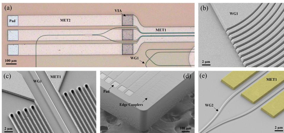
Fig. 4. (a) Optical microscope image of the TFLN PIC after the fabrication, (b) SEM image of a grating coupler patterned in WG1 layer, (c) SEM image of a thermo-optical phase shifter composed of a heater in MET1 layer and WG1 waveguide layer, (d) SEM image of a TFLN PIC encompassing a series of Pads for electrical probing and double-layer edge couplers for coupling to fibers, and (e) SEM image of an electro optical modulator in WG2 and MET1 layers (MET1 layer false-colored).
